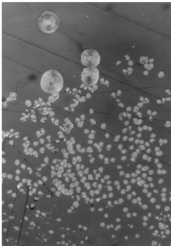
Figure 4 A polarized reflected light micrograph of cross section near surface of a PAN-based carbon fiber tow heat-treated at 2450 °C.
